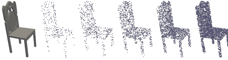
Figure 7: Point cloud sampling: input mesh, and point-clouds sampled with 256, 512, 1024, 2048, and 4096 points
