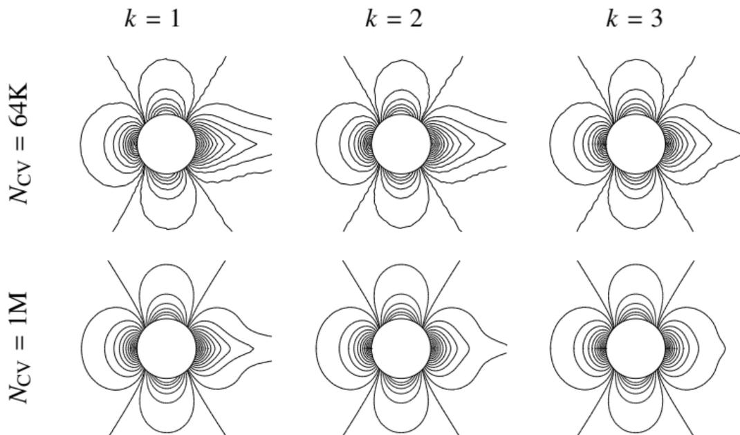
Computed Mach contours on the  $x_3 = 0$  symmetry plane for the sphere problem
