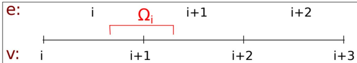
$$\left\{ \begin{array}{l} m_i \frac{dv_i}{dt} = -m_i(vv_x)_i + (\sigma_{i+1/2} - \sigma_{i-1/2}) + m_i g + O(\Delta x) \\ \frac{d\xi_i}{dt} = -(v\xi_x)_i \end{array} \right.$$
